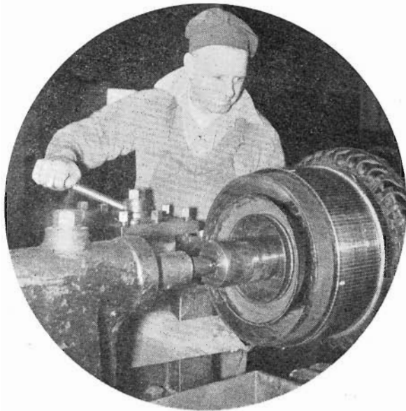
Truing up the commutator of an electric train motor.
