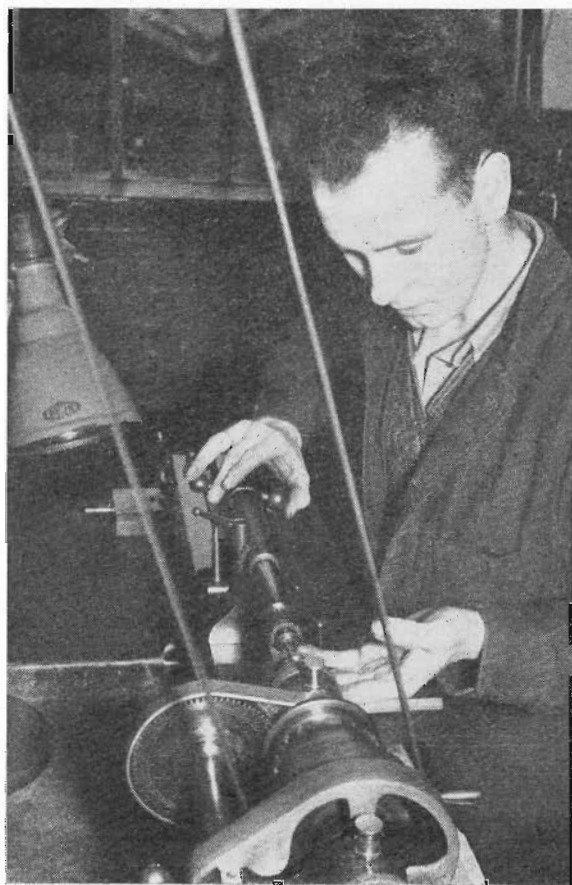
Fine work needs close concentration. The mechanic is turning a set of gauges to check the fuel jets in carburettors of petrol-electric cars.
